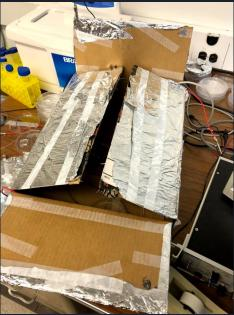
To reduce the room noise while recording samples, we used a carton box covered with aluminum foil.
